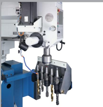
Automatic Tool Changing system (ATC) for 5 tools (Pos. 8.10) at the right side of the machine
