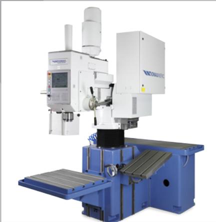
Angular table (Pos. 2.30) at the reverse side of the machine with swivable table (2.40) aside
