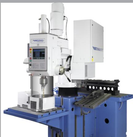
Angular table (Pos. 2.30) with workpiece at the reverse side, swivable table (Pos. 2.40) aside of the machine
