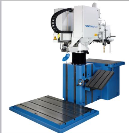
Floor Plate (Pos. 2.10) at the reverse side of the machine, with swivable table (Pos. 2.40) aside
