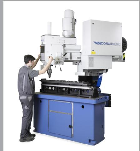
Manual operation, alternatively to the automatic CNC-mode-operation
